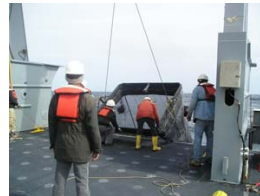
Japanese-designed midwater research trawl designed for towing at 4 – 5 kt for efficient capture of juvenile fishes and other micronekton.
